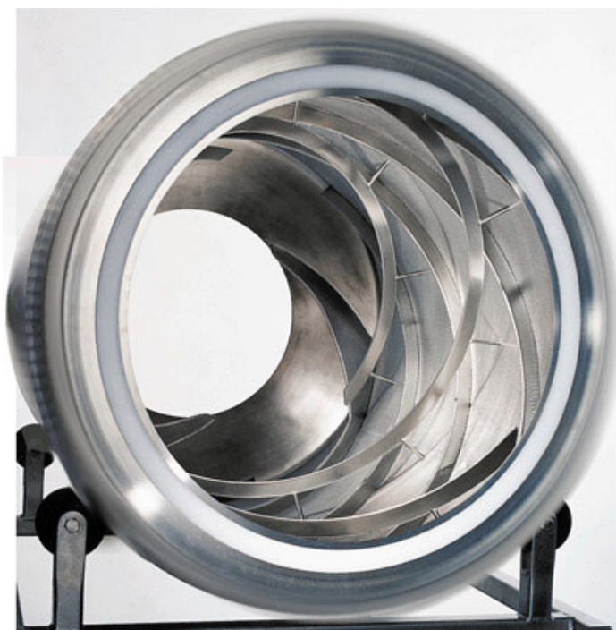
Figure 1. Coating drum with mixing ribbons.
